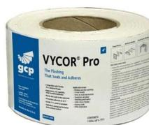
**Vycor PRO** flashing is composed of a durable, tear and puncture resistant engineered polypropylene backing film, paired with an aggressive, non-asphaltic, proprietary butyl-modified adhesive.
