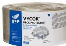
**Vycor Deck Protector** helps reduce corrosion of galvanized metal connectors. It is installed between the connector and the pressure-treated wood and acts as a barrier layer to break the electric circuit and thus helps reduce corrosion.
