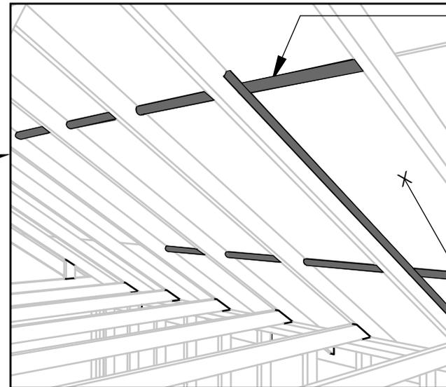
1.5" TO 3" FILLET OF 2-PART SPRAY-APPLIED CLOSED CELL POLYURETHANE FOAM ADHESIVE AT ALL JOINTS BETWEEN SHEATHING AND AT ALL INTERSECTIONS BETWEEN ROOF SHEATHING AND ROOF FRAMING MEMBERS, AND AT ALL VALLEYS. REFER TO MINIMUM REQUIREMENTS FOR SPRAY ADHESIVES.
