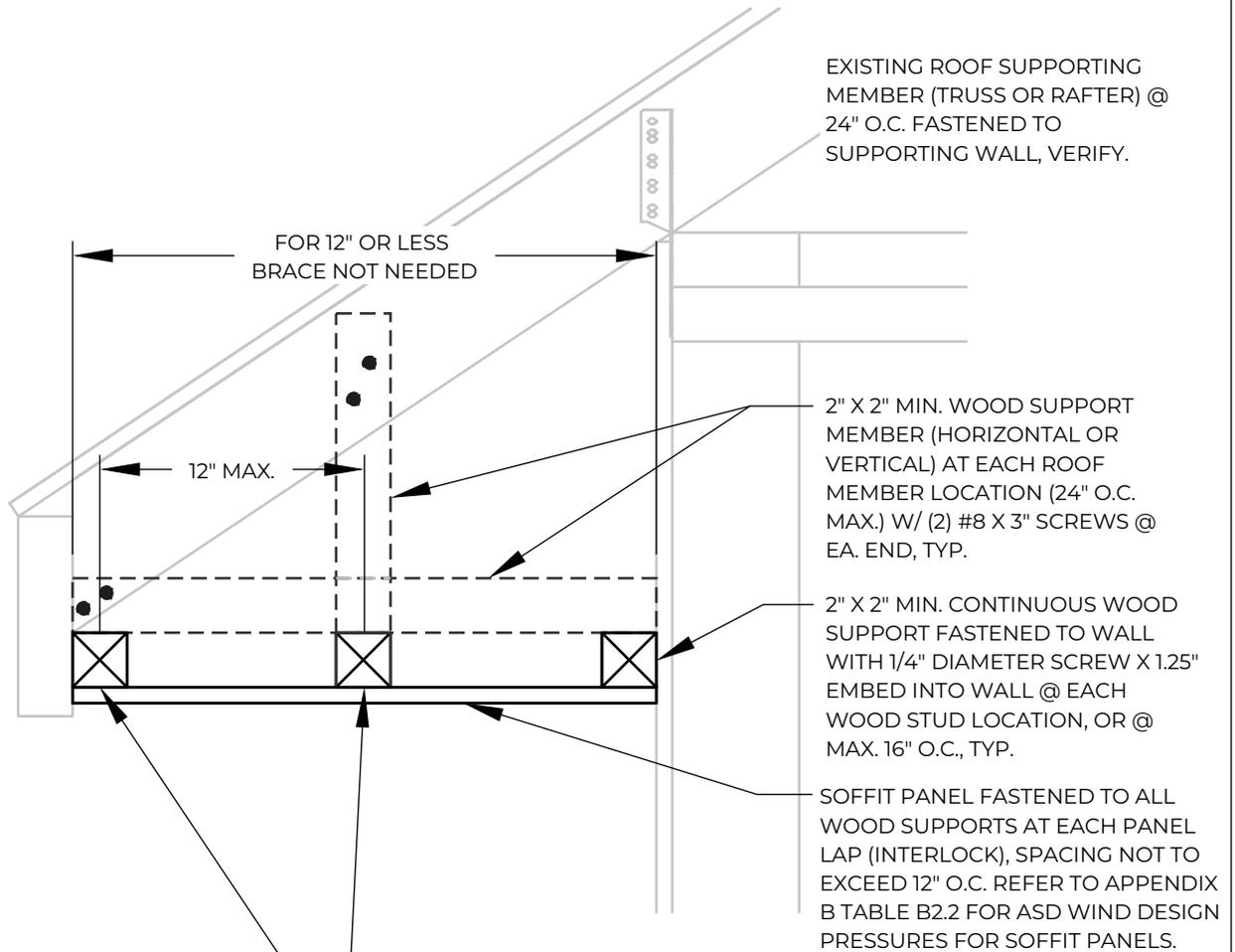
2" X 2" MIN. CONTINUOUS WOOD MEMBER SPACED @ MAX. 12" O.C. FASTENED TO WOOD SUPPORT W/ #8X3" SCREW AT EACH INTERSECTION, TYP.
