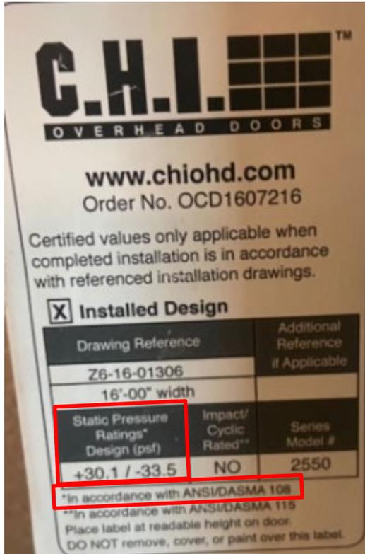
Figure 1. Photo of garage door label showing design pressure rating and test standard.
